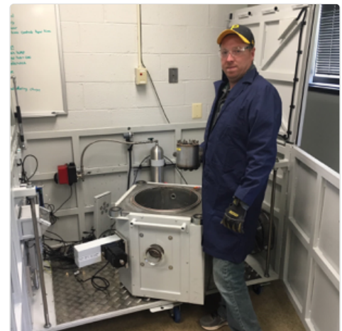
NIOSH technician with accelerating rate calorimeter (ARC).
