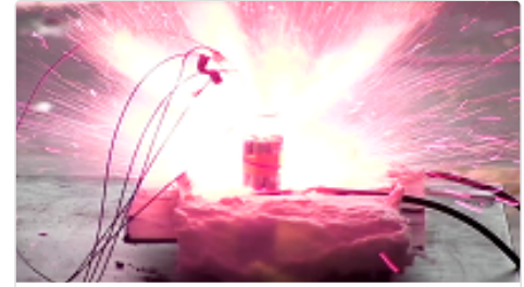
Figure 1. A lithium-ion battery pack undergoing thermal runaway. ( Click image for larger view )
