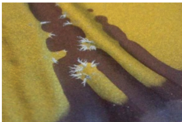
Figure 3. Lithium dendrites (white whiskers) created during repeated charge at low temperatures. Brown areas are un lithiated graphite (under the current collector fingers), and the gold color is lithiated graphite.
