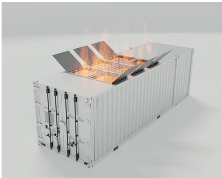
2. Explosion vent panels are installed on the top of battery energy storage system shipping containers to safely direct an explosion upward, away from people and property. Courtesy: Fike Corp.
